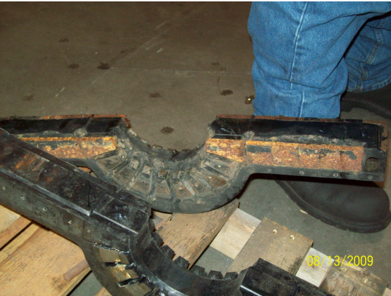
VBR elements; used (top), new (bottom)
